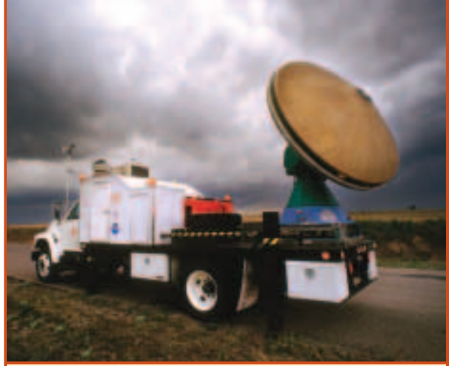
Mobile Doppler radar helps provide an early warning of severe weather.
